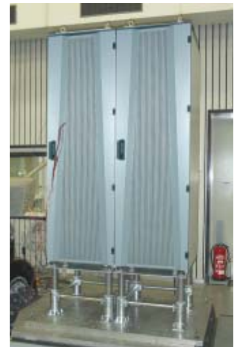
Dynamic seismic test in accordance with Bellcore Standard.
